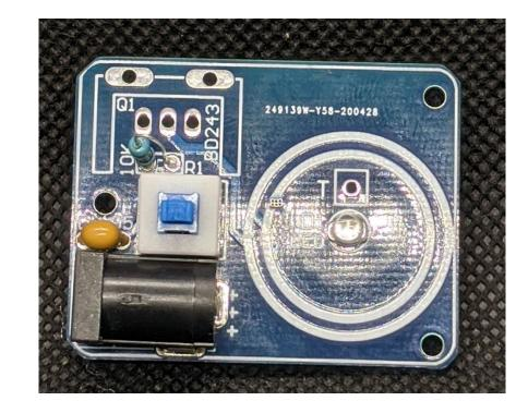
**4.** Solder the 1uF Capacitor, switch, and DC power jack as shown.
